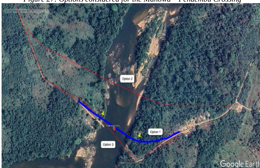
Figure 27: Options considered for the Manowa – Pendembu Crossing
